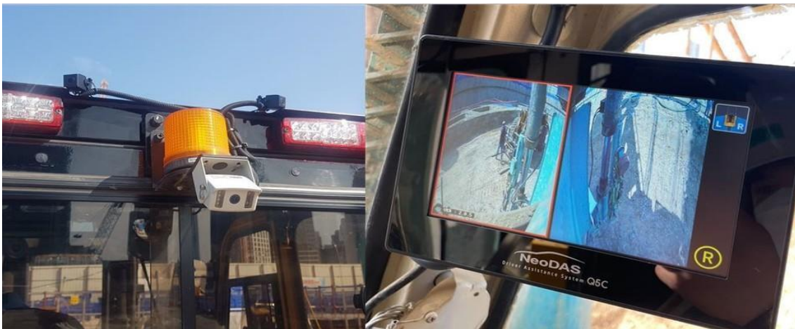
FIGURE E23: AI IMAGE RECOGNITION EQUIPMENT STENOSIS PREVENTION SYSTEM (SOURCE: PARK, 2023).
